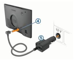
4 Plug the other end of the vehicle power cable (5) into a power outlet in your vehicle.
