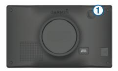
• To put the device in power saving mode, press the power key while the device is on.
